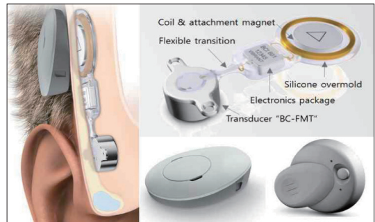
Fig. 11. Bonebridge (Photo courtesy MED-EL).
